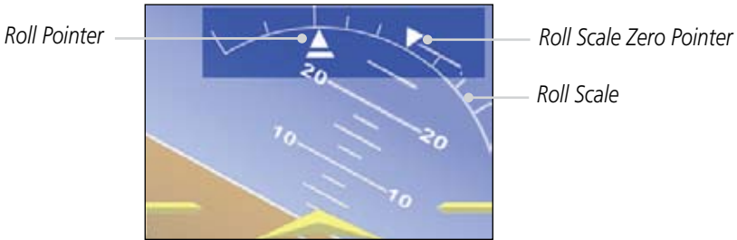
Figure 2-12 Attitude Indicator with a Ground Pointer configuration in a left turn
